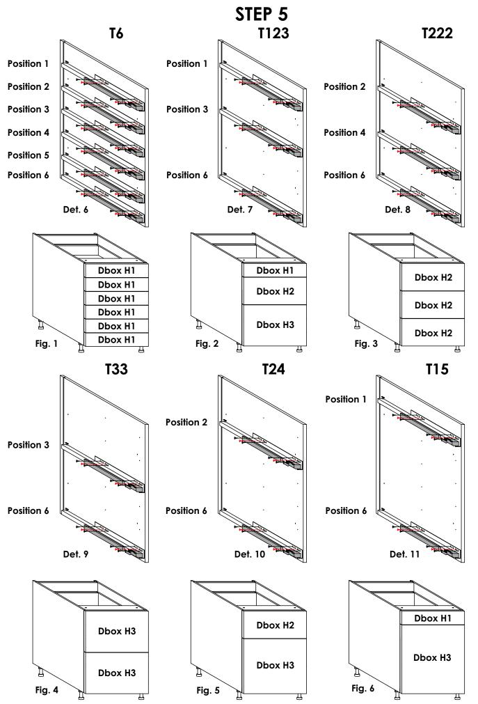
Using Screw 3.5 x 16mm, connect the Legrabox Runners to Panels A & B of the Drawer Cabinets. Confirm the desired configuration from Fig. 1-6 and connect the runners in the corresponding positions shown in Det. 6-11. The screws shown in red align with pre-drilled pilot holes. After fastening in the two screws in aligning positions, use four more screws to reinforce the runners as shown. Also, from fig. 1-6, note the specific Legrabox Drawer Box Heights that go into each configuration. BISON PG 4
