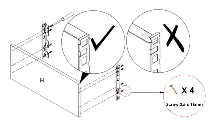
Place the Back Fixing Brackets in the shown positions on Panel H.
