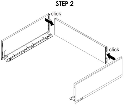
Connect the **Legrabox Drawer Sides** with panel **H** as shown. Do this by snapping the **Back Fixing** plates into the protrusions at the back of the **Drawer Sides**.
