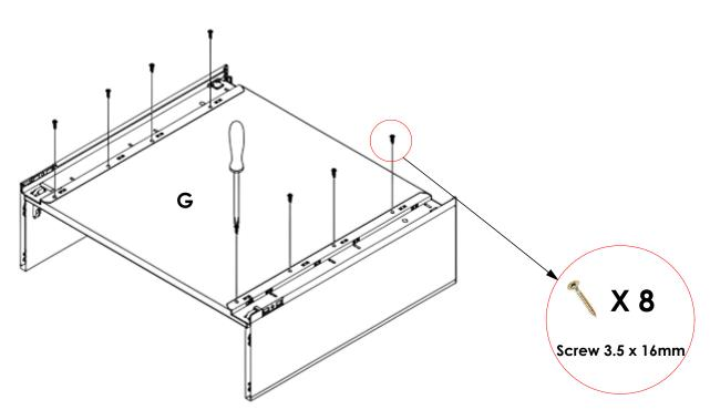
Using **Screw 3.5 x 16mm**, secure panel **G** in the shown positions.
