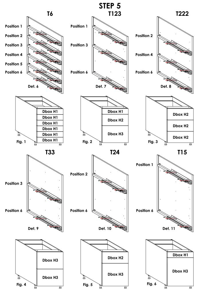
Using Screw 3.5 x 16mm, connect the Legrabox Runners to Panels A & B of the Drawer Cabinets. Confirm the desired configuration from Fig. 1-6 and connect the runners in the corresponding positions shown in Det. 6-11. The screws shown in red align with pre-drilled pilot holes. After fastening in the two screws in aligning positions, use four more screws to reinforce the runners as shown. Also, from fig. 1-6, note the specific Legrabox Drawer Box Heights that go into each configuration.
