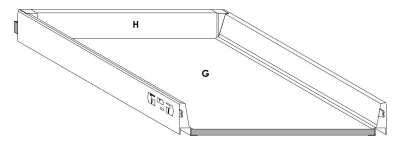
Confirm that the shaded edge on panel **G** is **flush** with the **front** of the **Antaro Drawer Sides**. If not, loosen the screws securing it and adjust accordingly.
