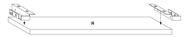
Place the Back Fixing Brackets in the shown positions on Panel H.
