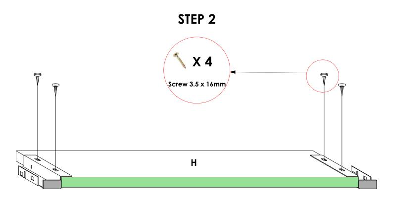
First, confirm that the shaded areas are **flush** with each other. Then, Secure the **Back Fixing Brackets** onto panel **H** using **screw 3.5 x 16** in the shown positions.
