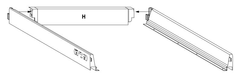
Connect the **Antaro Drawer Sides** with panel **H** as shown. Do this by snapping the **Back Fixing** plates into the protrusions at the back of the **Antaro Drawer Sides**.
