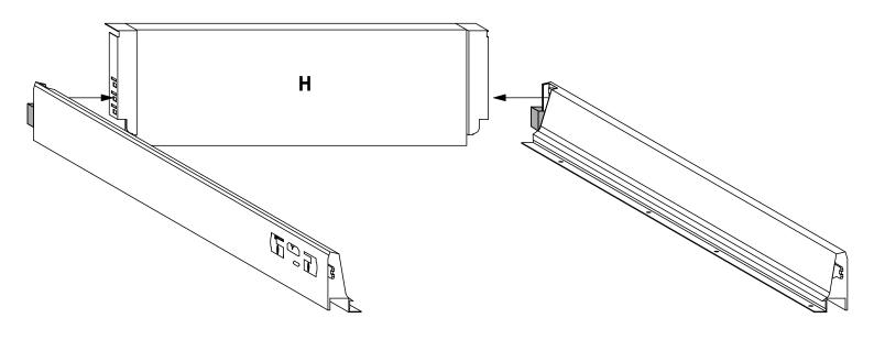
Connect the Antaro Drawer Sides with panel H as shown. Do this by snapping the Back Fixing plates into the protrusions at the back of the Antaro Drawer Sides.
