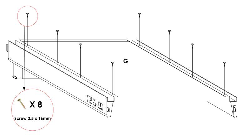
Using Screw 3.5 x 16mm, secure panel G in the shown positions.
