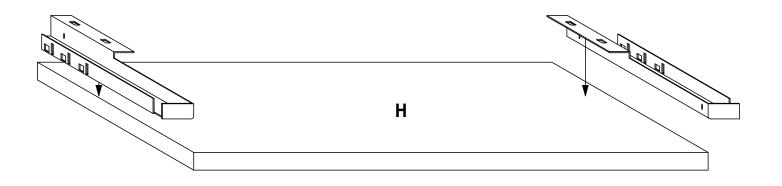
Place the Back Fixing Brackets in the shown positions on Panel H.
