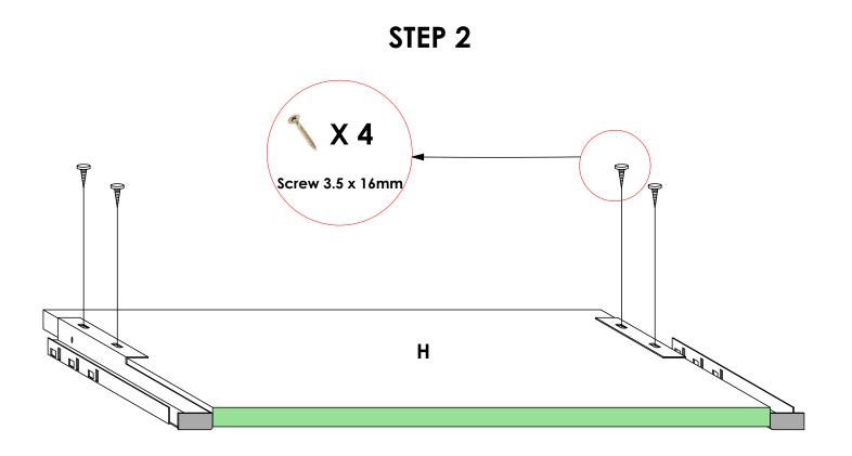
First, confirm that the shaded areas are **flush** with each other. Then, Secure the **Back Fixing Brackets** onto panel **H** using **screw 3.5 x 16** in the shown positions.
