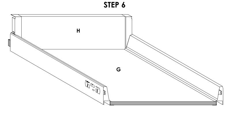
Confirm that the shaded edge on panel **G** is **flush** with the **front** of the **Antaro Drawer Sides**. If not, loosen the screws securing it and adjust accordingly.
