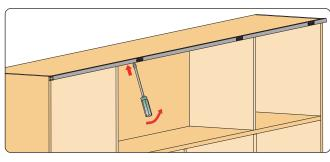
Slantly insert flathead screwdriver through the bottom track, until it gets close to connection piece, then pry open the track
