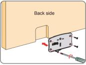
Install the stopper of damper in the middle of the panel of inner door
