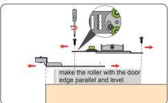
Adjust the door balance (adjust the bottom rollers)
