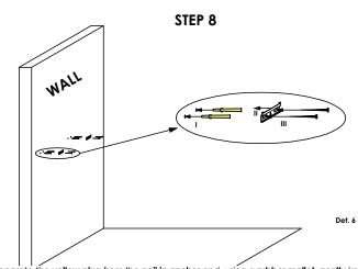
I) Separate the yellow plug from the nail in anchor and, using a rubber mallet, gently knock in the plug into the holes drilled in Step 5.
