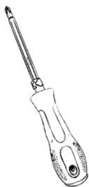
Screw Driver (Pozi Drive Head)
