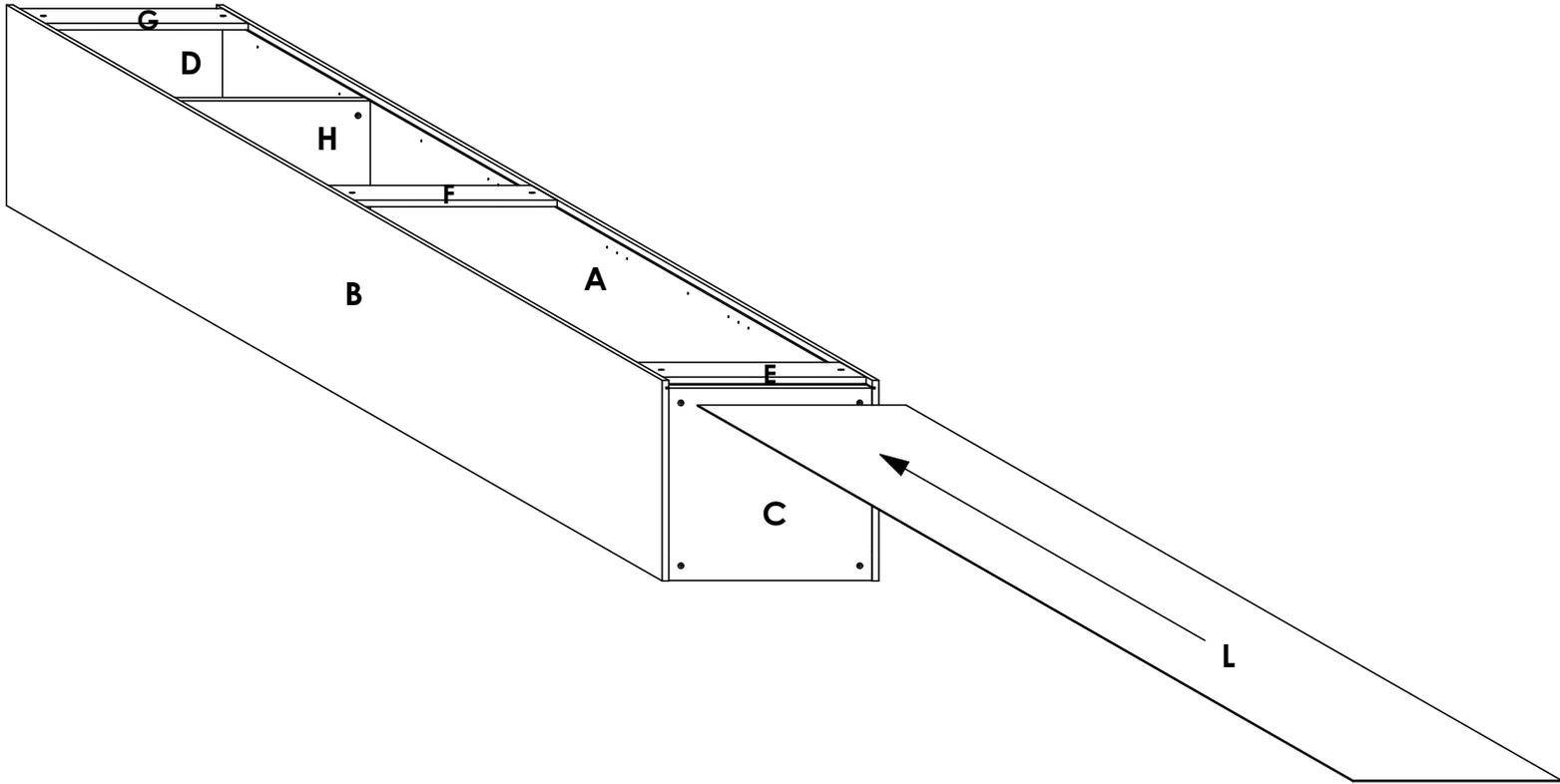
Slide the 3mm panel (L) into the groove on panels A & B with the finished side facing down. Refer to the holes and/or grooves on the diagram to determine the panel orientation.
