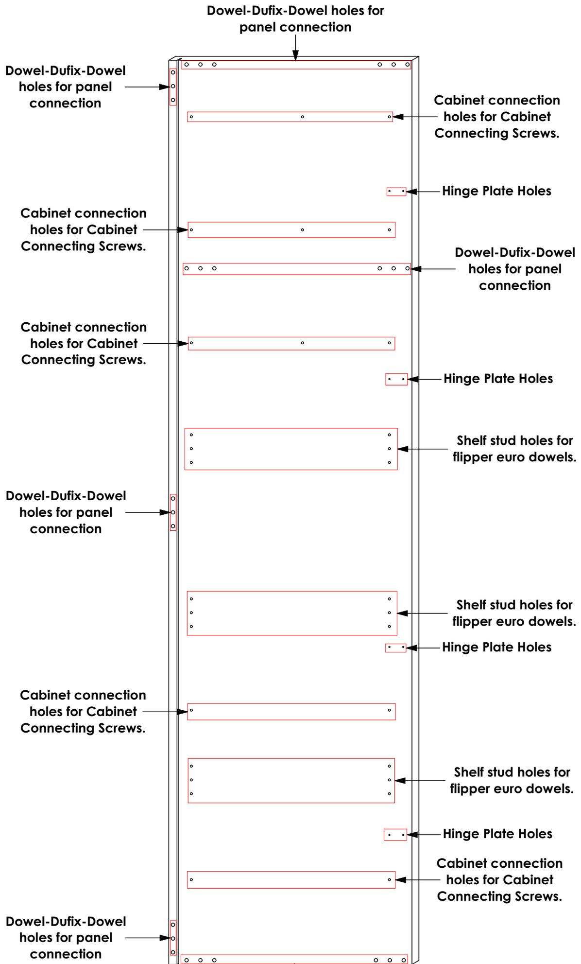
Dowel-Dufix-Dowel holes for panel connection
