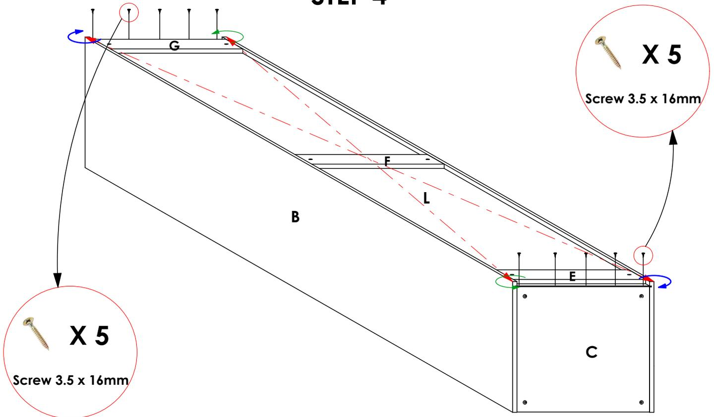
First, **check the diagonal** of the cabinet by measuring the two distances indicated by the broken lines. They should be equal. If not, twist the cabinet accordingly in the diagonal corners as shown until an equal value is achieved. After, secure panel F to panels C & D as shown using **Screw 3.5 X 16mm**.
