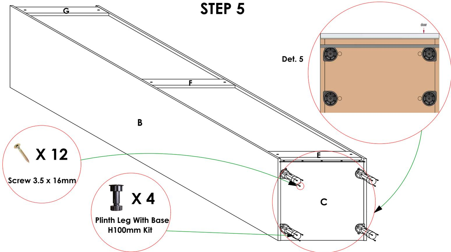
Place the four units of **Leg Adjustable Base 100mm** in the shown positions, aligning with the pre-drilled pilot holes on panel **C**. Ensure that the orientation is as shown in **Det. 5**. Using **Screw 3.5 X 16mm**, secure the legs onto panel **C**.
