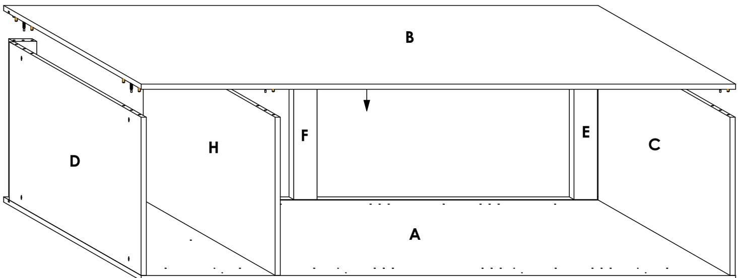
Connect panel **B** to panels **C, D, E, F, G & H** as shown. Refer to the holes and/or grooves on the diagram to determine the panel orientation.
