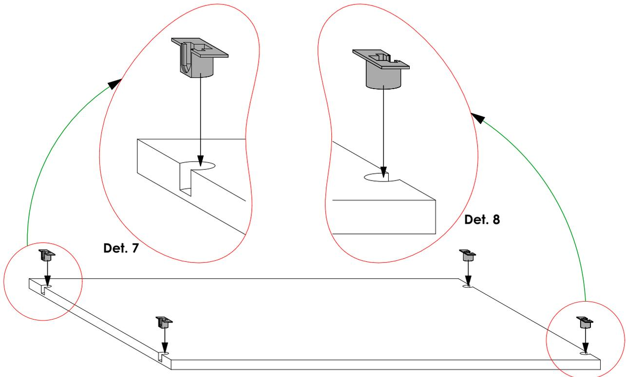
Insert the **shelf supports** for flipper in the shown positions on panels **I, J & K**. Confirm that the orientation is as shown in **Det. 7** and **Det. 8**.
