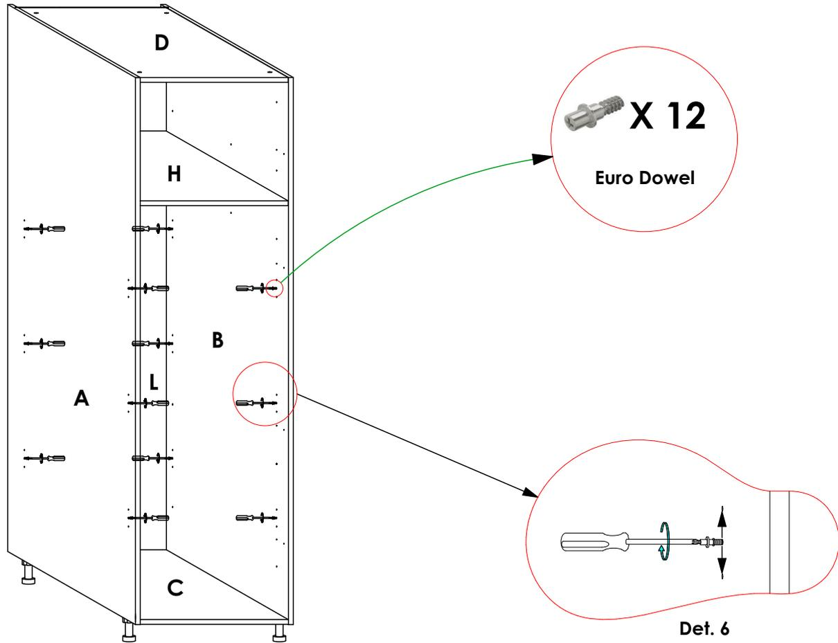
Screw in the **Euro Dowels** for flipper in the shown positions. Their positions can be adjusted as shown in **Det. 6** to change the level of the shelves or to slant the shelves.
