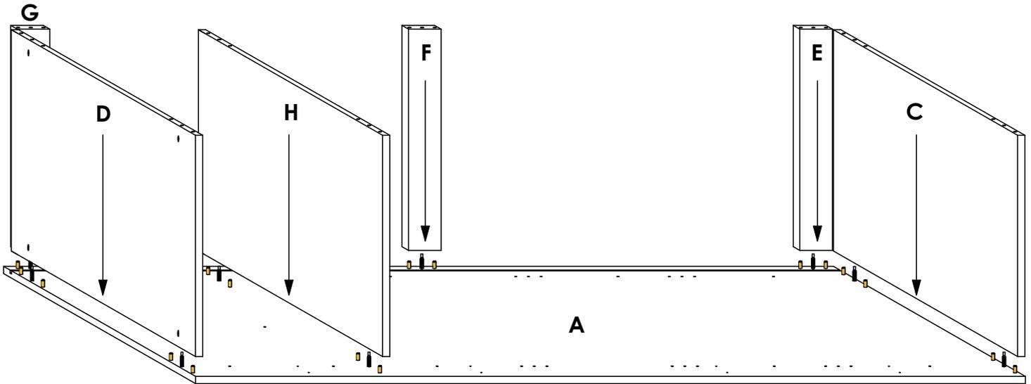
Connect panels **C, D, E, F, G & H** to panel **A** as shown. Refer to the holes and/or grooves on the diagram to determine the panel orientation.
